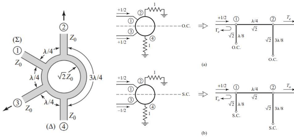
Derive the following ABCD parameters for the figures (a) and (b).
