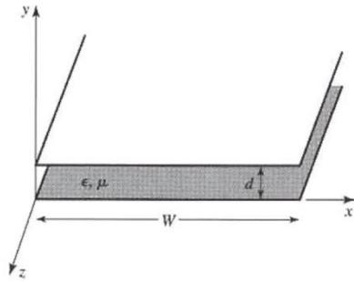
7. Consider the following the parallel plate waveguide. Assume that the strip width  $W$  is much greater than the separation  $d$ . A material with permittivity  $\epsilon$  and permeability  $\mu$  is assumed to fill the region between the two plates. Find  $H_x(x,y,z)$  and  $E_y(x,y,z)$ . (Assume that  $k^2 = \omega^2 \mu \epsilon$  and  $E_z(x,y,z) = e_z(x,y)e^{-j\beta z}$ )
