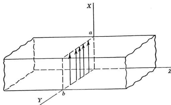
6. Consider the following the parallel plate waveguide. Assume that the strip width  $W$  is much greater than the separation  $d$ . A material with permittivity  $\epsilon$  and permeability  $\mu$  is assumed to fill the region between the two plates. Find  $E_z(x,y,z)$ . (Assume that  $k^2 = \omega^2 \mu \epsilon$  and  $E_z(x,y,z) = e_z(x,y) e^{-j\beta z}$ )
